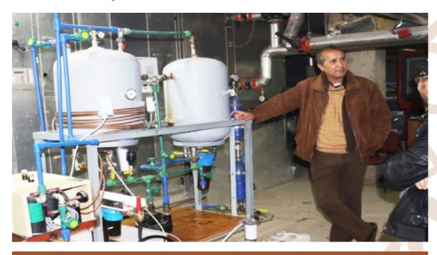
A project funded by an AUI Seed Money Grant has developed a small-scale converter which processes used cooking oil into biodiesel fuel. In contrast to large, expensive systems, this converter uses mostly recycled materials. Tests show that it produces cleaner fuel and also allows the users to collect byproducts such as glycerin which can be used for other purposes.
